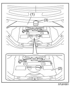
The jack wheel brace and jack handle are stowed in the luggage under-box (2) under the trunk floorboard (1). The floorboard can be kept raised using the hook (3).
